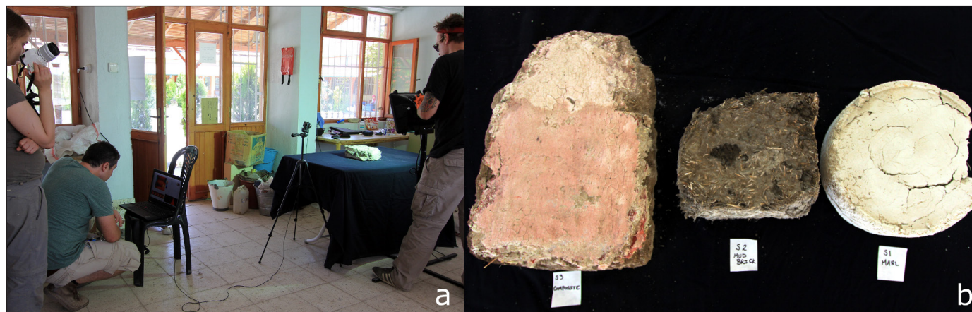
Figure 2. View of (a) Çatalhöyük Digital Preservation Team performing experimental thermal infrared imaging in the Conservation Lab and (b) analogue mudbrick with pigmented plaster, analogue mudbrick, and natural marl samples used in the experiment.
