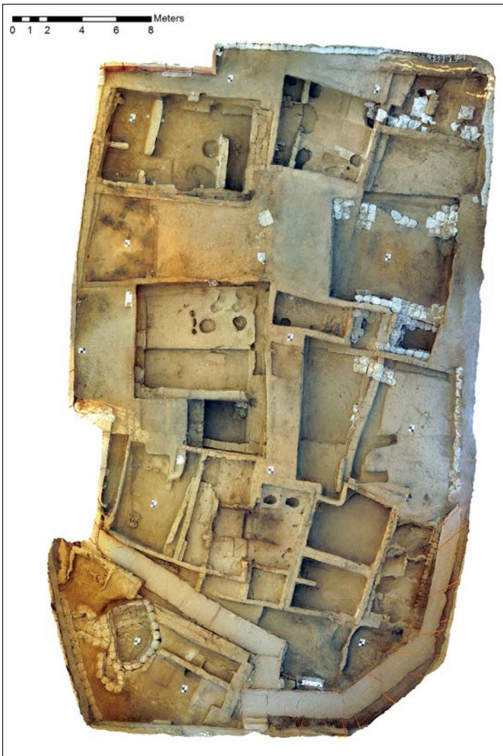
Fig. 21.2. Orthomosaic of the North Area in 2015 generated using UAV imagery georeferenced using Ground Control Points from the Çatalhöyük survey team.
