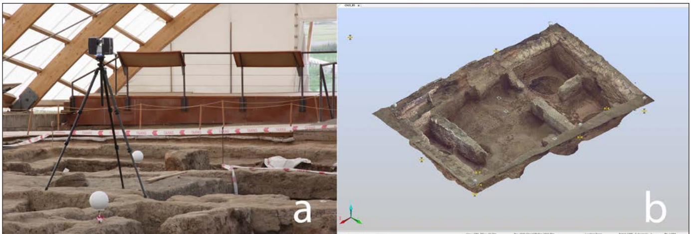
Fig. 21.1. View of (a) FARO Focus 3D S120 unit scanning the North area in 2012 and (b) post processed point cloud of B.5 in 2015.
