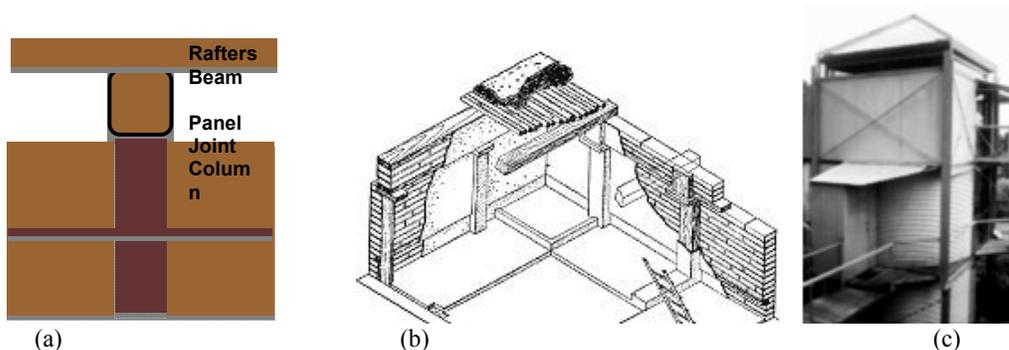
Figure 136 Principles of the Structural System: (a) Inferred Mellaart roof beam section; (b) Reconstruction of typical Çatal building Level VI (Mellaart, 1967 in Hodder, 2005); (c) External steel frame tower (Ganis, 1998)
