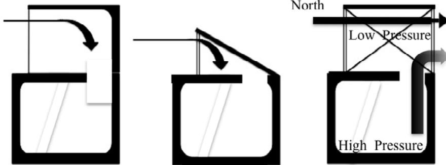
Figure 135. Mounded settlement (above); rooftop shelters and the effect on prevailing wind (below): (a) Cutting (2005); (b) Düring (2000); (c) Proposed breeze-way rooftop shelter structure.
