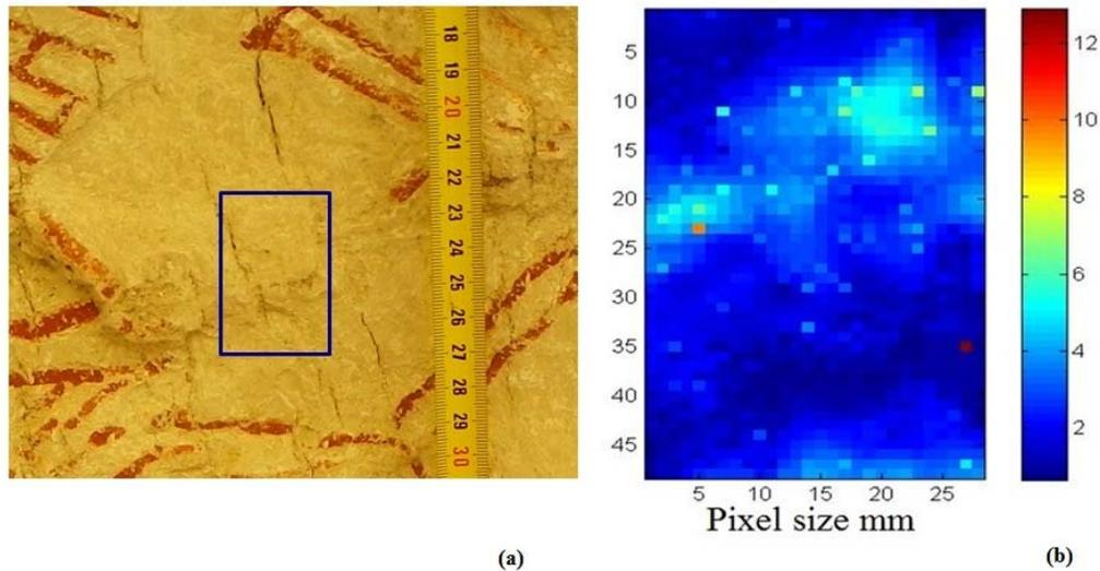
Figure 174. (a) Photograph of a section of wall painting from the South Area, Room 80 with the scanned section highlighted. (b) a reconstructed sub-surface image of the highlighted area of the wall.
